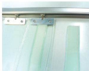
Fasten the end of sheet to the frame with hook-and-loop fastener (width 50mm) when closed-for single leaf
