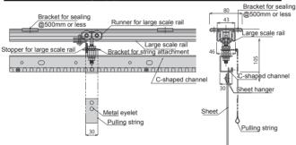
Weight: Approx.2.8kg per meter (not including the weight of the sheet)
