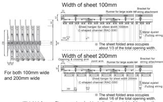
Weight: Approx.5kg per meter (not including the weight of the sheet)
