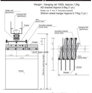
% The sheet folded area occupies about 1/4~1/5 of the total opening width. Weight: Approx.5kg per meter (not including the weight of the sheet)
